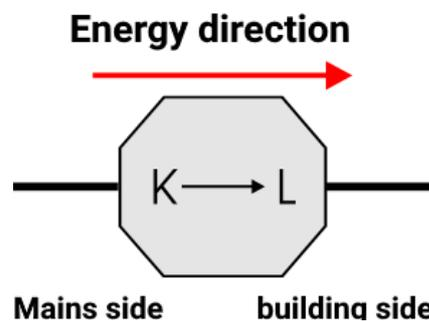
Each current transformer must be closed carefully by clicking the snap fastener securely into place. If the energy direction is changed, the energy meter counts in the negative.
