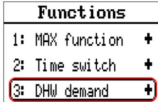
The function **DHW demand** is selected. Ensure that the name of the function and not the plus symbol next to it is highlighted with a box around it.
