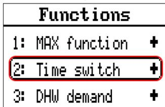
The function **Time switch** is selected. Ensure that the name of the function and not the plus symbol next to it is highlighted with a box around it.
