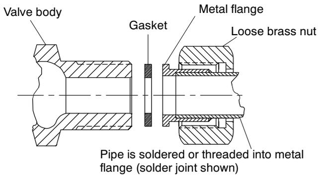
Pipe is soldered or threaded into metal flange (solder joint shown)
