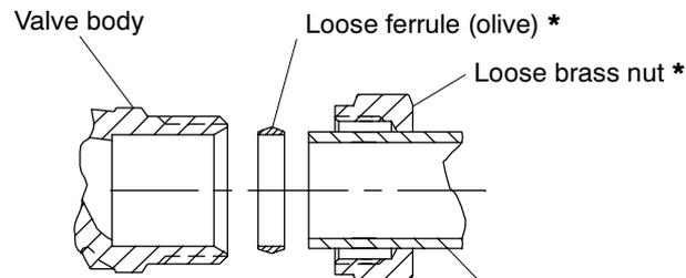
Using ferrule and nut for sealing 22 mm outerdiameter pipe.
