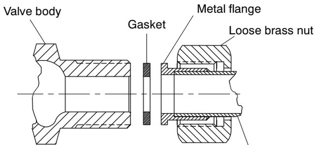
Pipe is soldered or threaded into metal flange (solder joint shown)
