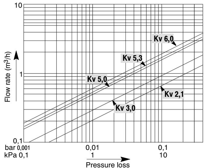
**Fig. 7. Valve pressure loss characteristic for 2-way valves**
