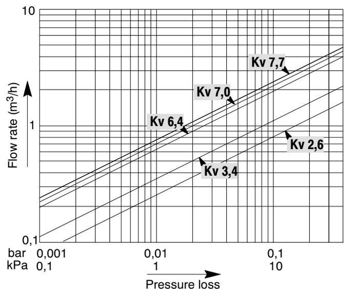
**Fig. 8. Valve pressure loss characteristic for 3-way valves**
