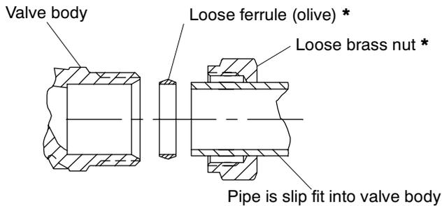
Pipe is slip fit into valve body
