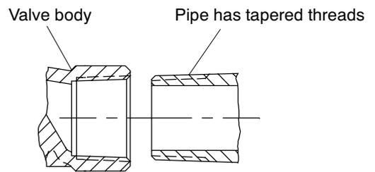
**Fig. 31. 1" BSPT internal (Rc 1) or 1" NPT internal**
